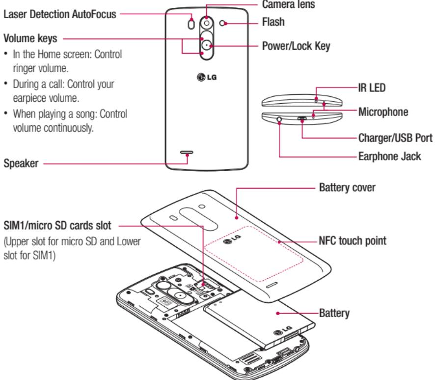
**LDAF Sensor (Laser Detection AutoFocus Sensor)** : By detecting the distance with laser, when you recording with the rear camera lens, LDAF Sensor enables you to focus the long or close range more fast and accurately.
